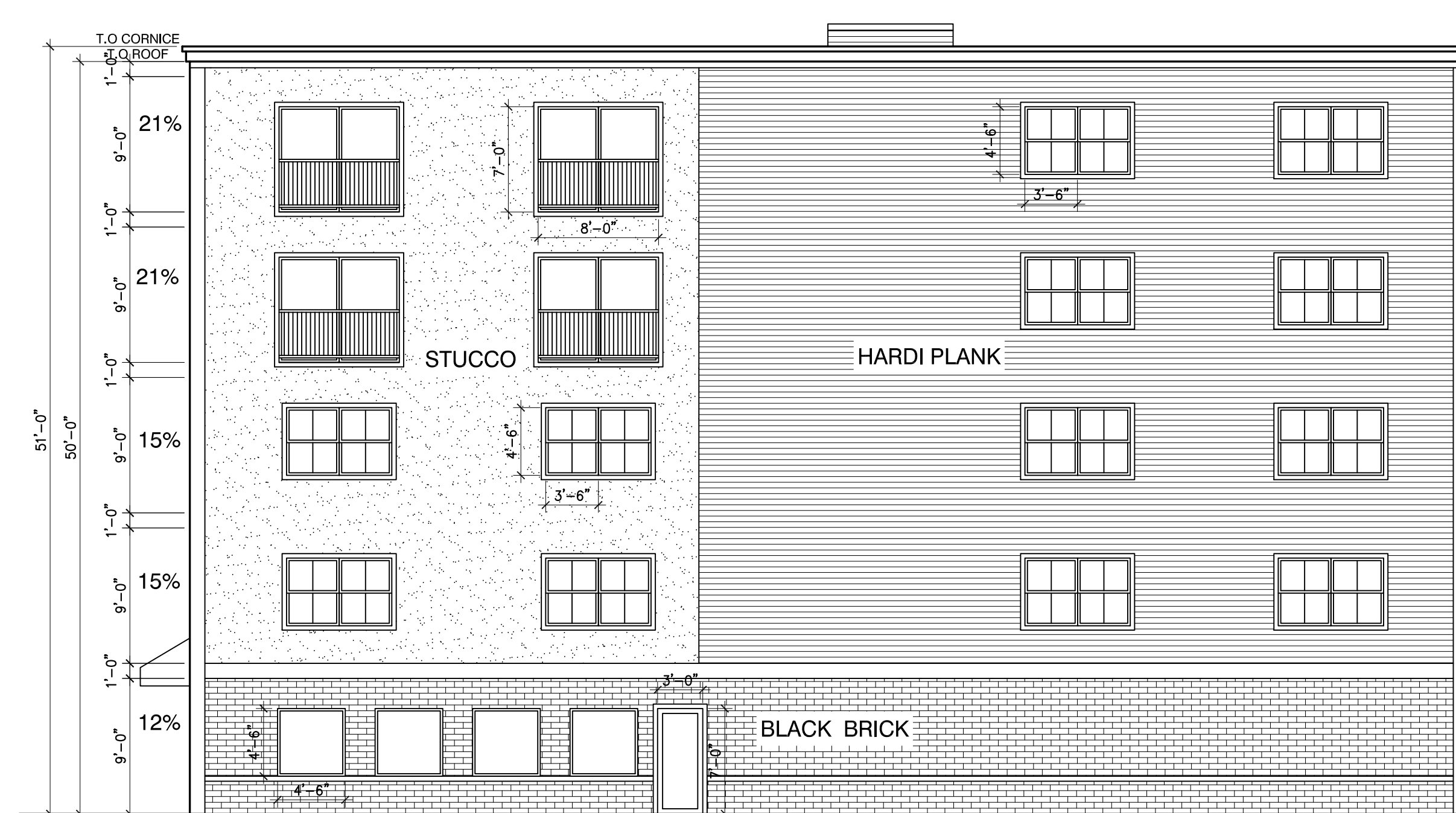
4 A2 LOT 3C PROPOSED NORTH ELEVATION 1/8"=1'-0"
